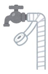
• If your pipes do freeze, open the faucet and wrap the part of the pipe that is frozen with a towel, and pour warm water over it. (If you pour boiling or hot water directly over the pipe, causing it to heat too quickly, this can cause the pipe to burst) If water still won't come out of the pipe, contact a plumber. If you live in an apartment, contact the landlord of the building or real estate company. It will cost money to repair.
